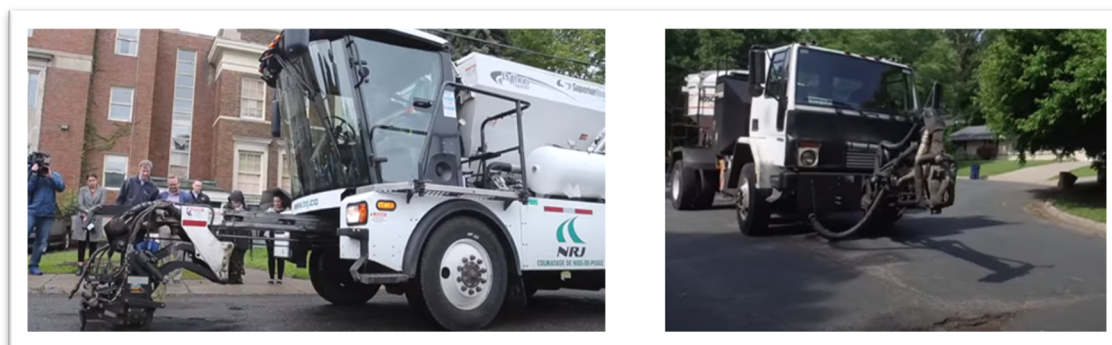
Figure 29. Semi-automatic potholes repairs
