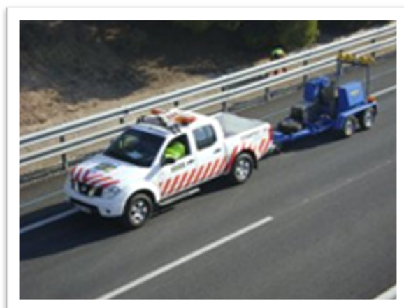
Figure 23. Tow impact deflectometer
