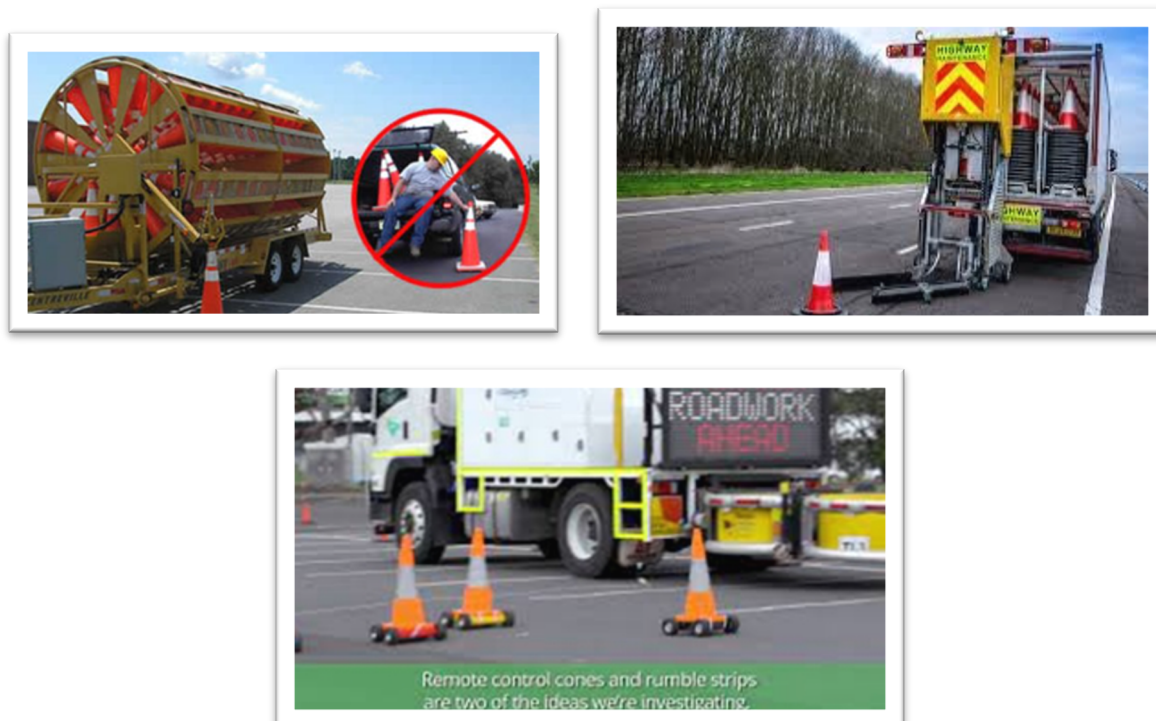
Figure 36. Advanced systems to limit the human intervention associated to the use of cones
