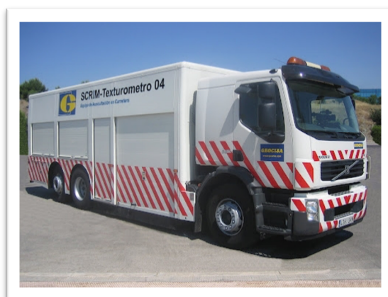
Figure 22. SCRIM skid testing machine for texture measurements
