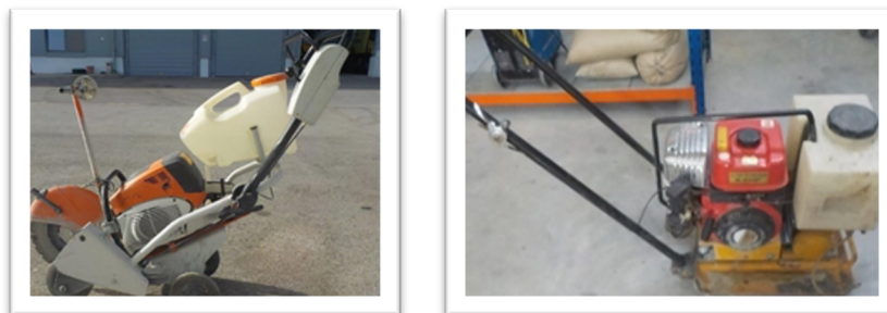
Figure 31. Asphalt cutter and vibrating/compaction plate
