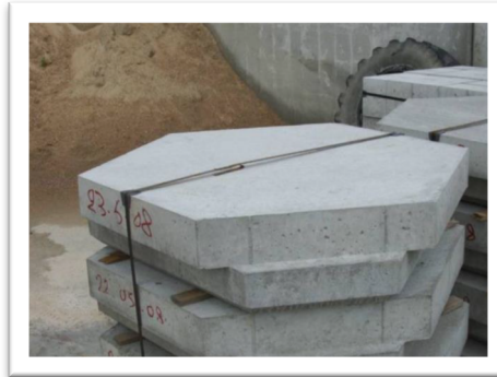
Figure 17. RUP slab with connectors
