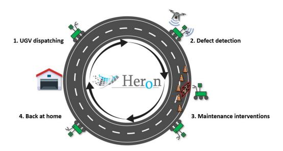
HERON aims to develop an integrated automated system to perform maintenance and upgrading roadworks tasks, such as sealing cracks, patching potholes, asphalt rejuvenation, autonomous replacement of CUD elements and paint markings, but also supporting the pre-/post-intervention phase, including visual inspections and dispensing and removing traffic cones in an automated and controlled manner.
