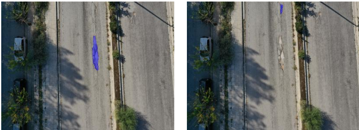
Figure 12: Pothole segmentation from UAV data using YOLO v8 and SAM
