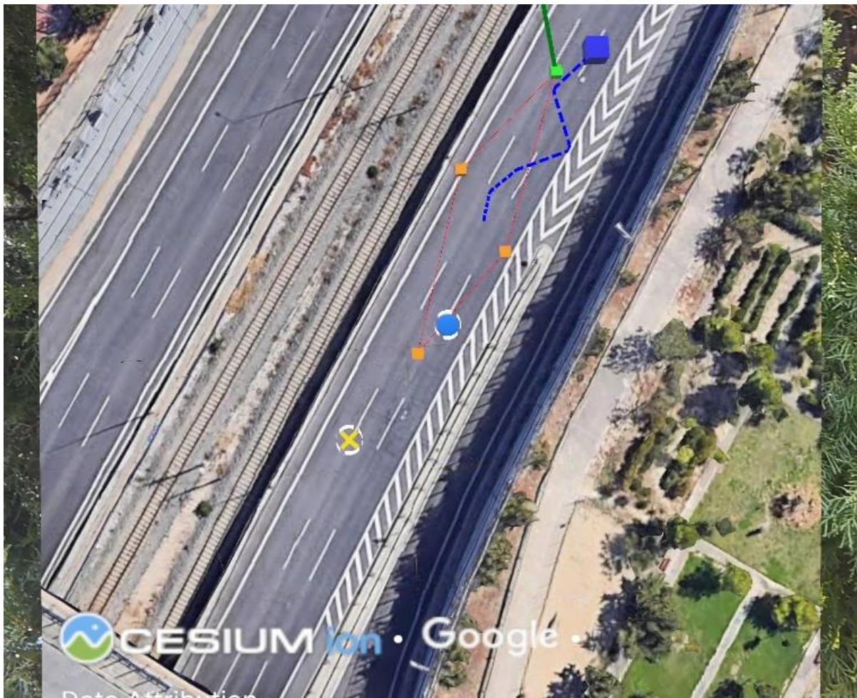
Figure 7: Example of visualization of the robot's position (blue rectangle) and trajectory (blue dash line) on the satellite map.
